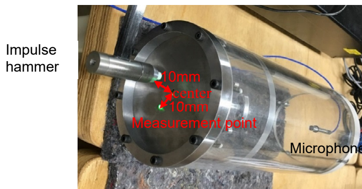
Fig. 4. Excited point and measurement point
