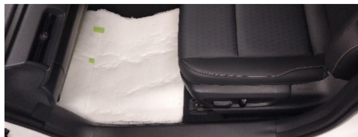
Fig. 8. Added sound absorption material (PET : thickness 50mm).
