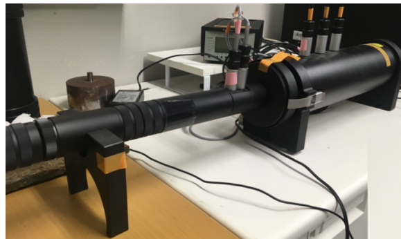
Fig.1. Experimental setup using acoustic pipe.
