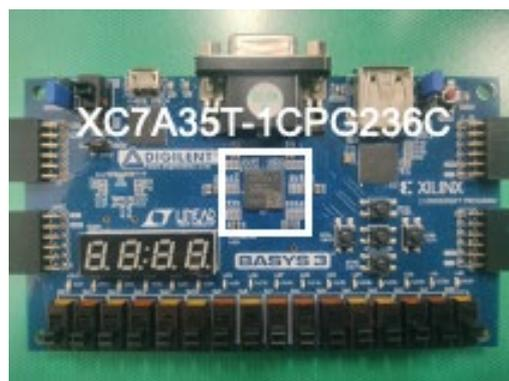
Fig. 8. Experimental environment: Zoomed Basys 3 Artix-7 FPGA board.
