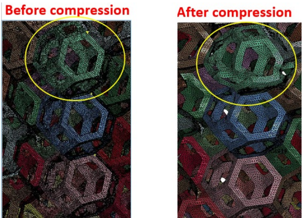
Fig. 9. Nonlinear elastic deformation before / after compression of microscopic multiple Kelvin cells in Urethane foam.
