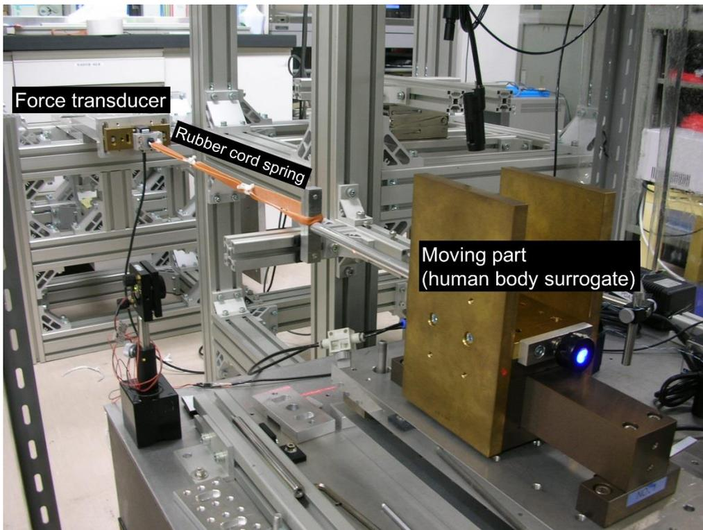
Fig. 2. Photograph of the experimental setup
