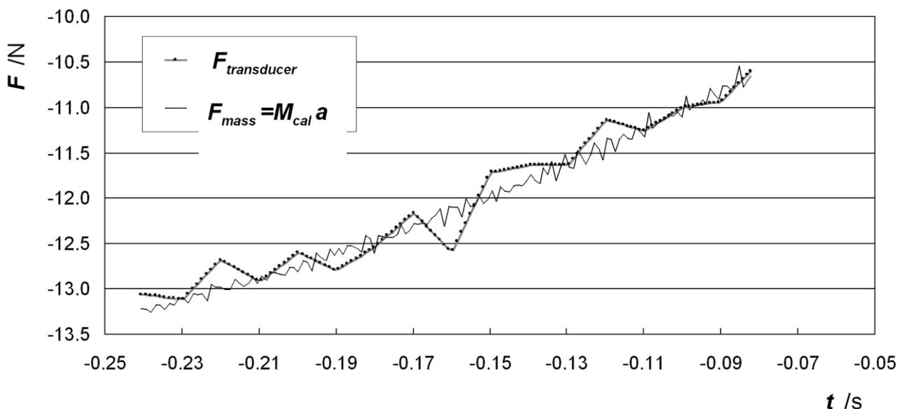
Fig. 3. Force measured using force transducer and optical interferometer
