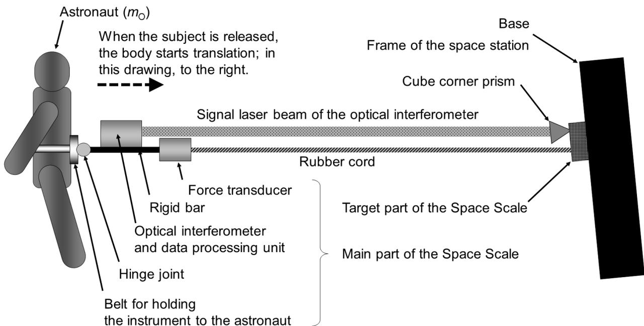
Fig. 4. Space Scale for Astronaut Mass Measurement
