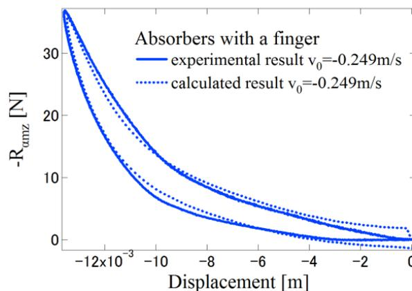
Fig. 6 Hysteresis curves of a pair of viscoelastic shock absorbers with a finger from FEM
