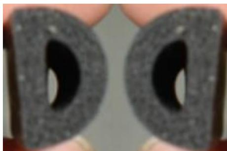
Fig. 1 A pair of viscoelastic shock absorbers
