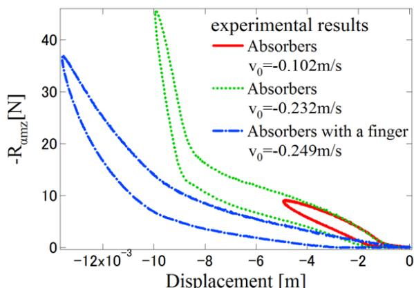
Fig.3 Experimental results of restoring forces for viscoelastic shock absorbers
