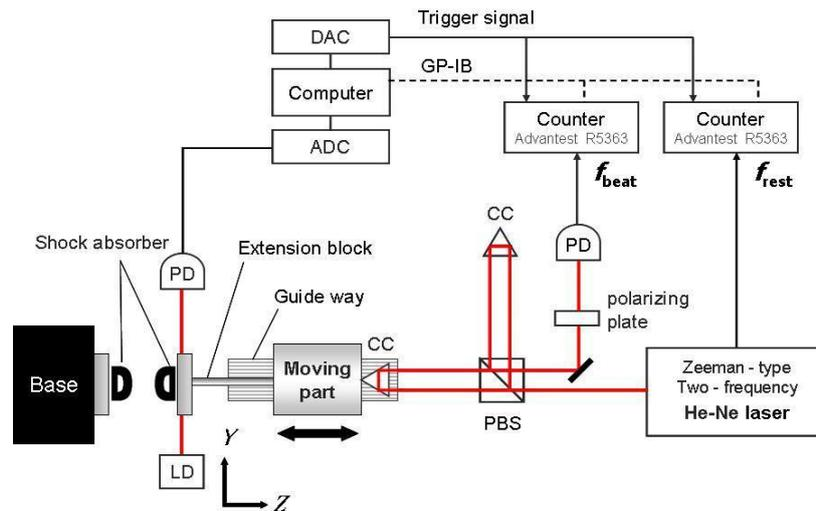
Fig.2 Experiment setup [7]
