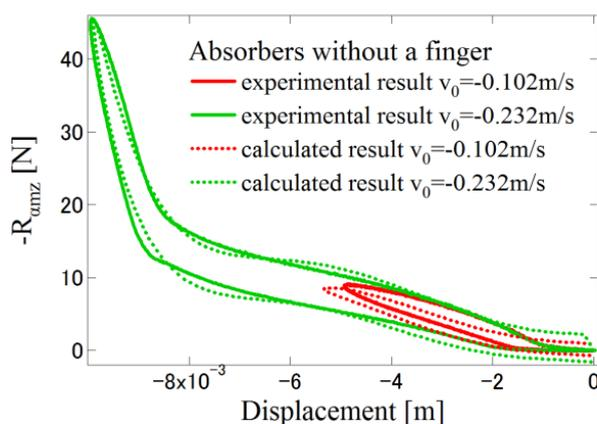
Fig. 5 Hysteresis curves of a pair of viscoelastic shock absorbers without a finger from FEM
