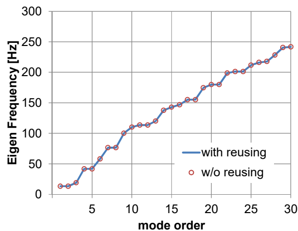
Fig.7 Eigenfrequency Computed with/without the Reuse Procedure.
