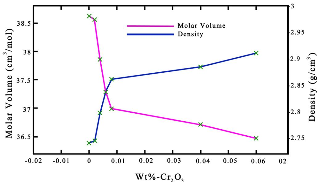
Fig. 8. Relation of the density and molar volume with Cr<sub>2</sub>O<sub>3</sub> wt% for zinc sodium phosphate (NZP) glass system.
