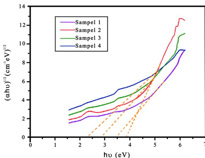
Fig. 5. The Gap Energy Value Determination.
