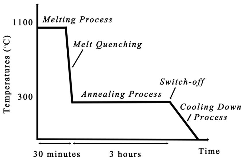
Fig. 1. Glass Making Process Temperature.
