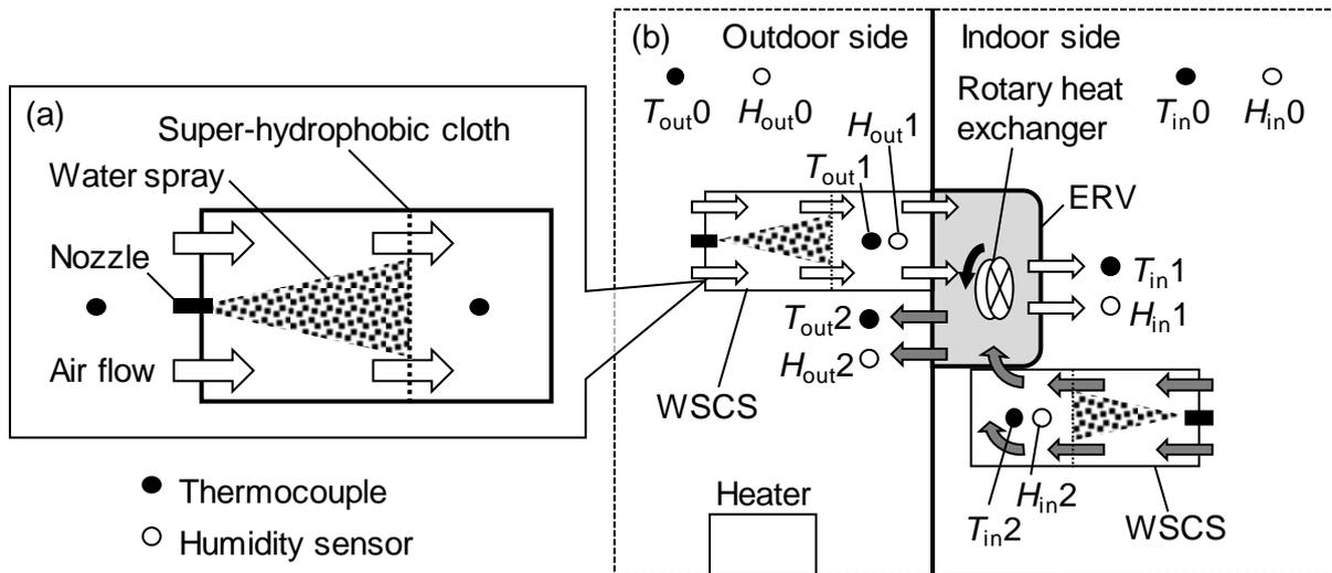
Fig. 2. (a) WSCS and (b) experimental apparatus
