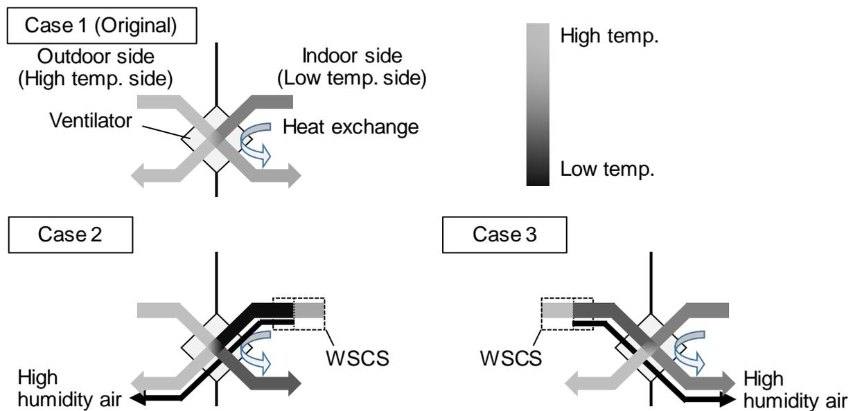
Fig. 1. Concept of ERV with WSCS
