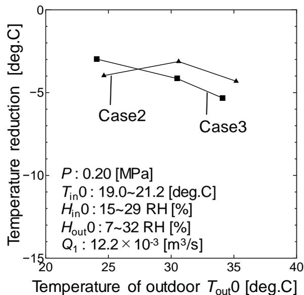
Fig. 3. Temperature reduction by water spray
