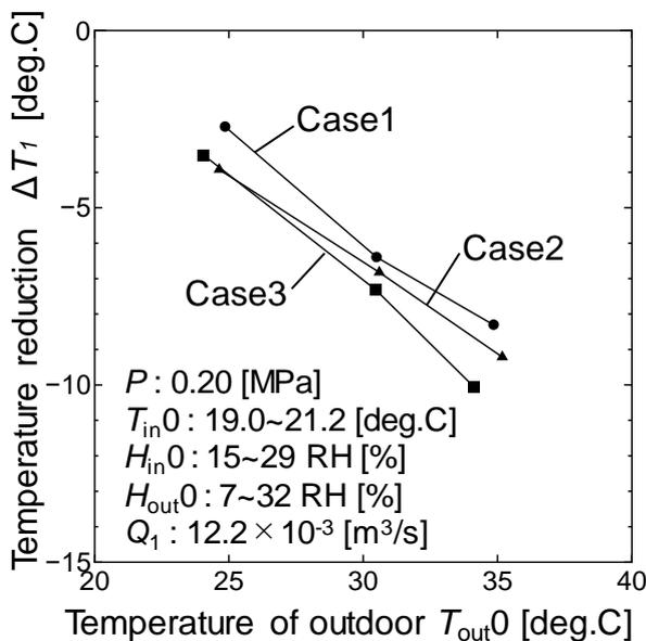
Fig. 6. Effect of outdoor temperature on temperature reduction
