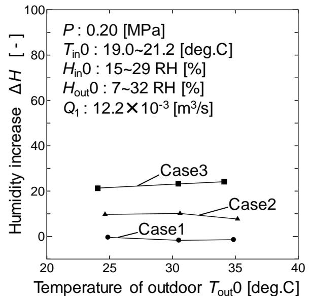
Fig. 7. Effect of outdoor temperature on humidity increase
