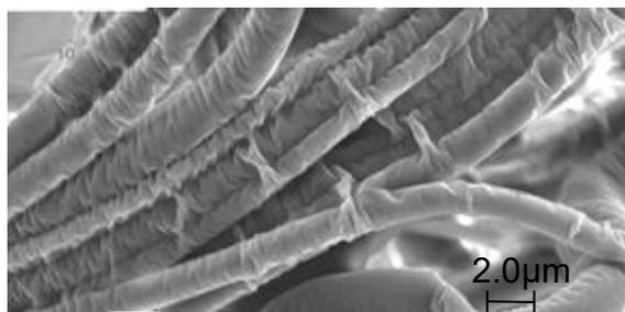
Fig. 1 Ultrafine fibers (fiber diameter : about  $2.0 \mu\text{m}$ )
