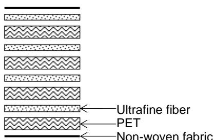
Fig. 4 Sound absorption material laminating pattern
