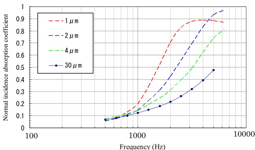
Fig. 2 Sound absorption coefficient of fibers ( $300 \text{ [g/m}^2\text{]}$ , thickness:  $10 \text{ [mm]}$ )
