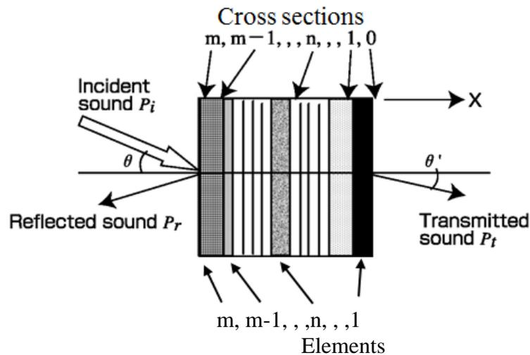
Fig. 3 Model of sound insulation material
